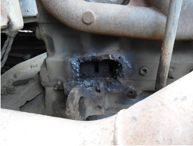
Engine: 5” hole in engine block
