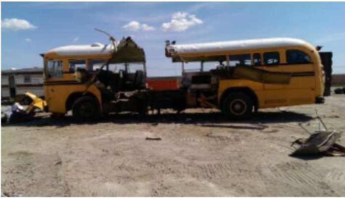
Example of acceptable destruction of vehicle chassis
